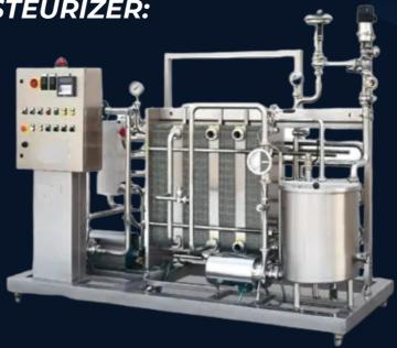
To improve the safety and shelf life of milk, this milk pasteurizer is the perfect solution. Its designed to kill harmful bacteria, pathogens and microorganism in milk by heating. This pasteurizers were capable to process huge volumes of raw milk and equipped with advanced control systems like temperature control systems to achieve desired level of pasteurization, user-friendly control panel, safety sensors and emergency stop buttons to ensure safety.
