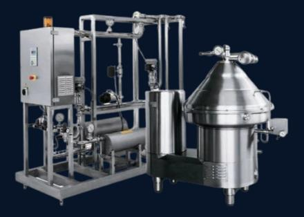
The clarifier works by utilizing centrifugal force it separates the heavier particles from the milk such as dirt, dust & other impurities are forced to the outside of the rotating bowl.
