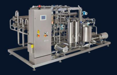
Milk filtration machine involves in milk processing plant that removes impurities & solid particles from the raw milk to produce a safe and quality milk. Firstly, the raw milk passed through a series of filters which removes large particles like dirt, hair & insects. Then passed through finer filters which removes bacteria, somatic cells & other impurities.
